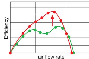
Several hundred propeller shapes are put to trial calculation to select the shape with best efficiency.
